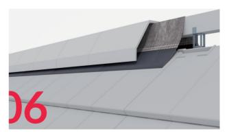
Every ridge and hip tile should be fixed using a clamp. The clamps should be screwed in using stainless steel screws.
