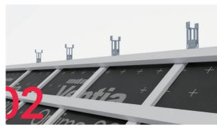
Install the battens. The batten spacing depends on the roof tile model applied. The installation of battens should be started from the eaves line. The sub-ridge batten should be fixed in the distance of 3.5-4.5 cm from the roof top.
