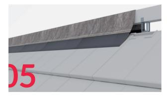
After laying the last row of roof tiles the ridge tape should be unwound and fixed (e.g. by means of staples, with 1 m spacing) directly onto the ridge batten. The edges of ridge tape should be profiled properly and then glued tightly to the roof tiles (the roof tiles should be cleaned properly). The minimum overlap of tape and roof tiles is 50 mm. In case it is necessary to combine two ridge tapes, there should be applied an overlap of at least 75 mm.
