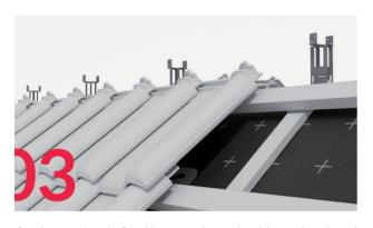
On the previously fixed battens there should now be placed the roof tiles in accordance with the fundamental principles of roofing.
