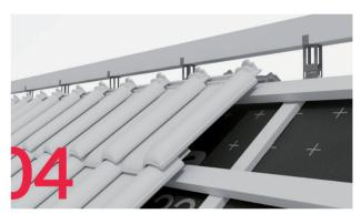
On the grip attached there should be placed and screwed in the ridge batten.
